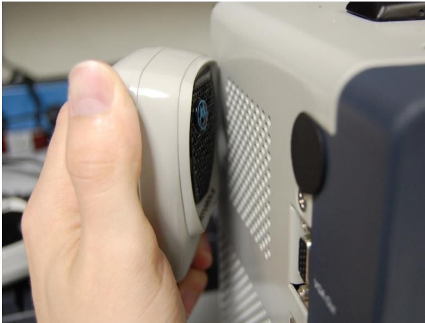
Figure 6-2. Place keyed microphone next to analyzer speaker.
