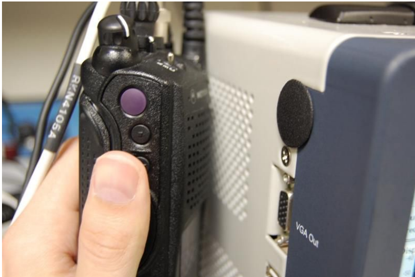
Figure 4-1. Place keyed radio next to analyzer speaker.
