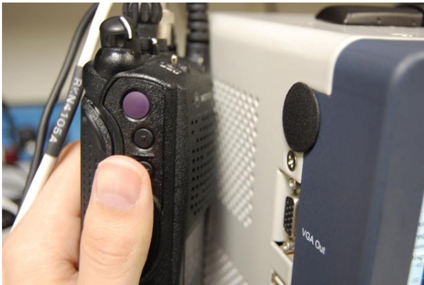
Figure 6-1. Place keyed radio next to analyzer speaker.
