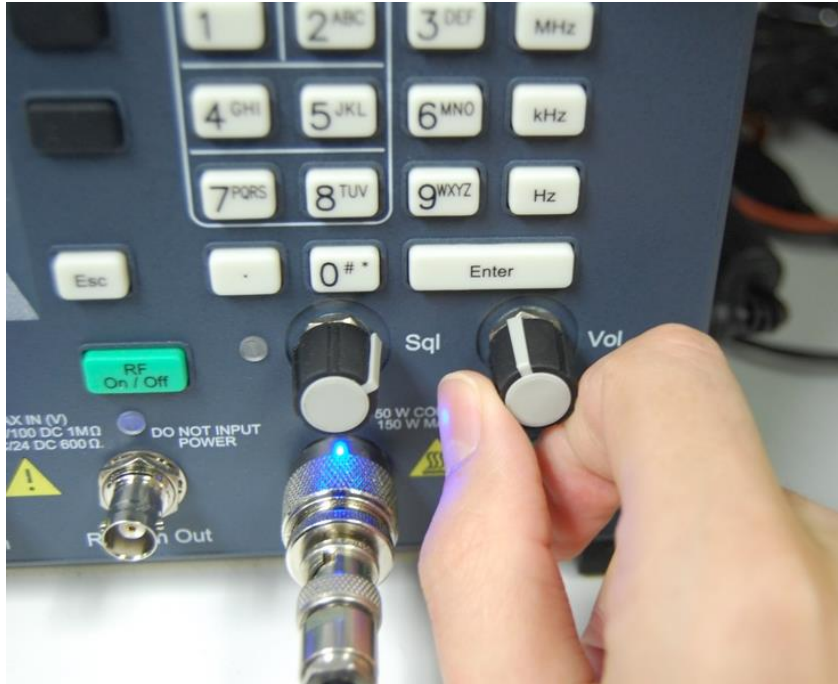
Figure 6-2. Adjust analyzer volume until about 4 kHz deviation is measured.
