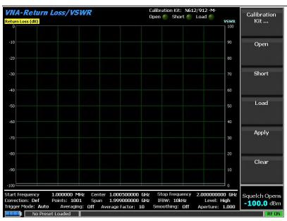
This selects the N612/912-M calibration kit and returns to the Calibration display.
