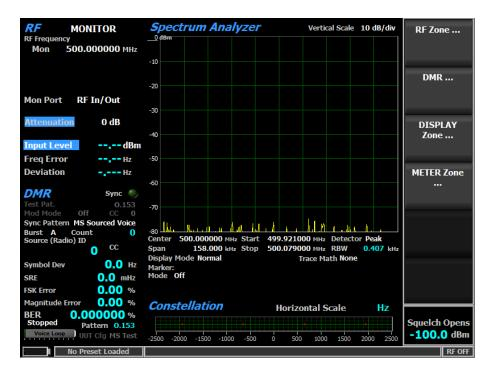
Pressing **Test** > **Test Mode** > **DMR** configures the R8200 for DMR protocol testing, as shown above. The default mode's AUDIO Zone and associated soft keys on the R8200 display are replaced by the DMR Zone and DMR-specific soft keys (accessed by pressing the **DMR** soft key).
