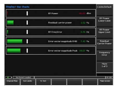
The full screen Bar Charts Display include soft keys for configuring the Test Limits of the measurements represented in the Bar Charts Display.
