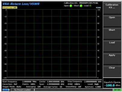
This enters the other half of the data necessary to calculate phase error associated with your transmission line into the calibration data set.
