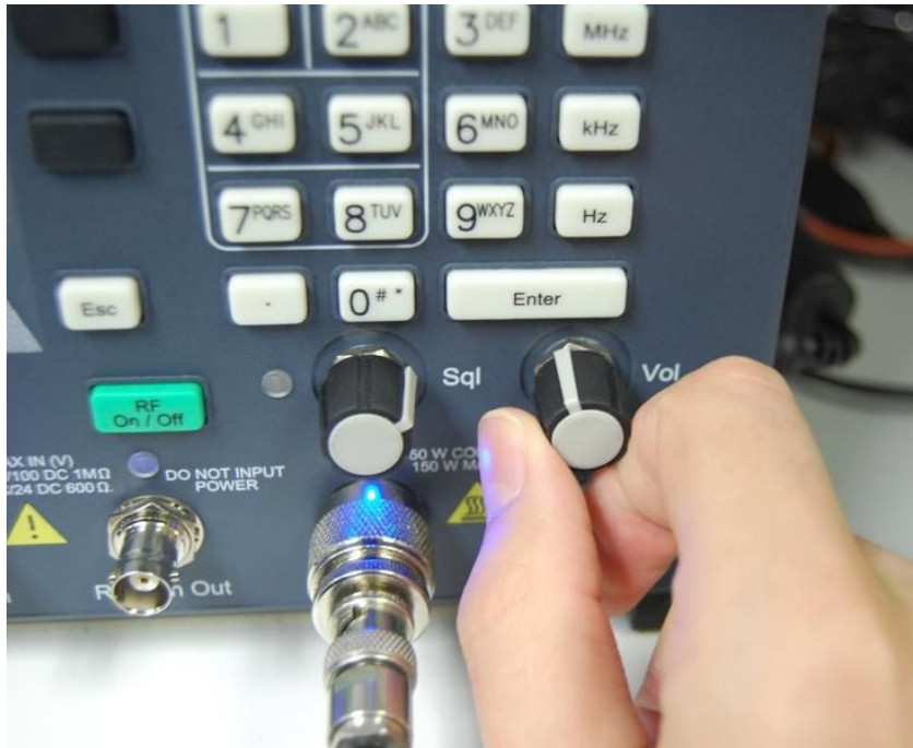
Figure 6-3. Adjust analyzer volume until about 4 kHz deviation is measured.
