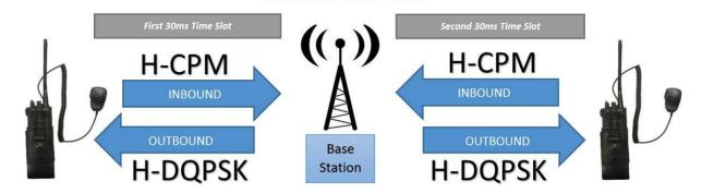
P25 Phase 2 voice channels are 12.5 kHz wide and contain two time slots. Each slot carries a separate channel of traffic. This means the portable/mobile radio is only transmitting 50% of the time.
