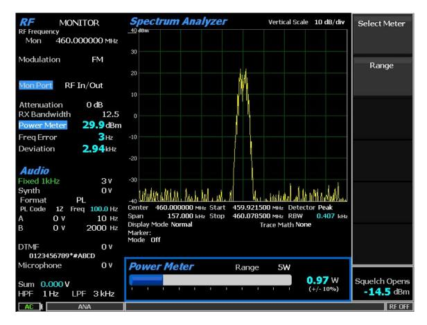
**Note 2:** The R8000 configuration and settings above may be saved as a "Preset". This avoids having to go through the above procedure every time you need to conduct this test.
