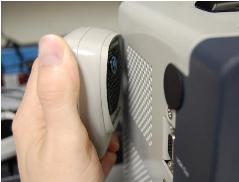
Figure 6-2. Place keyed microphone next to analyzer speaker.
