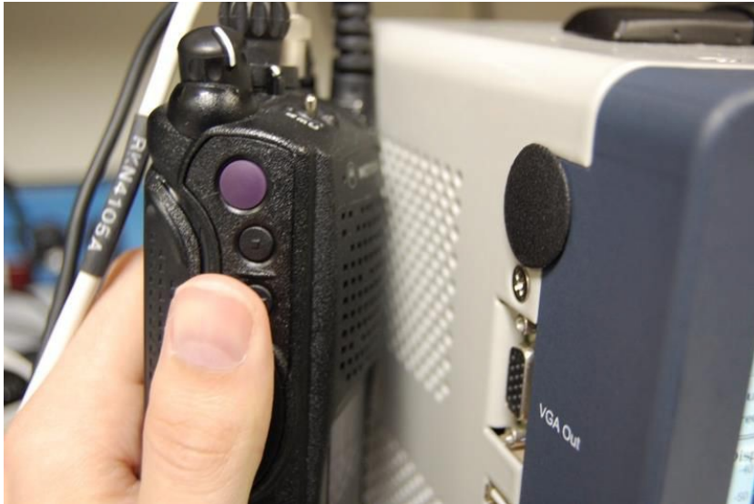
Figure 4-1. Place keyed radio next to analyzer speaker.
