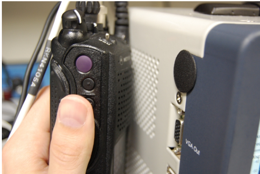
Figure 4-1. Place keyed radio next to analyzer speaker.
