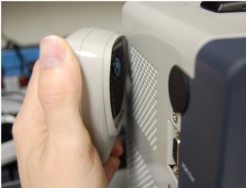
Figure 6-2. Place keyed microphone next to analyzer speaker.
