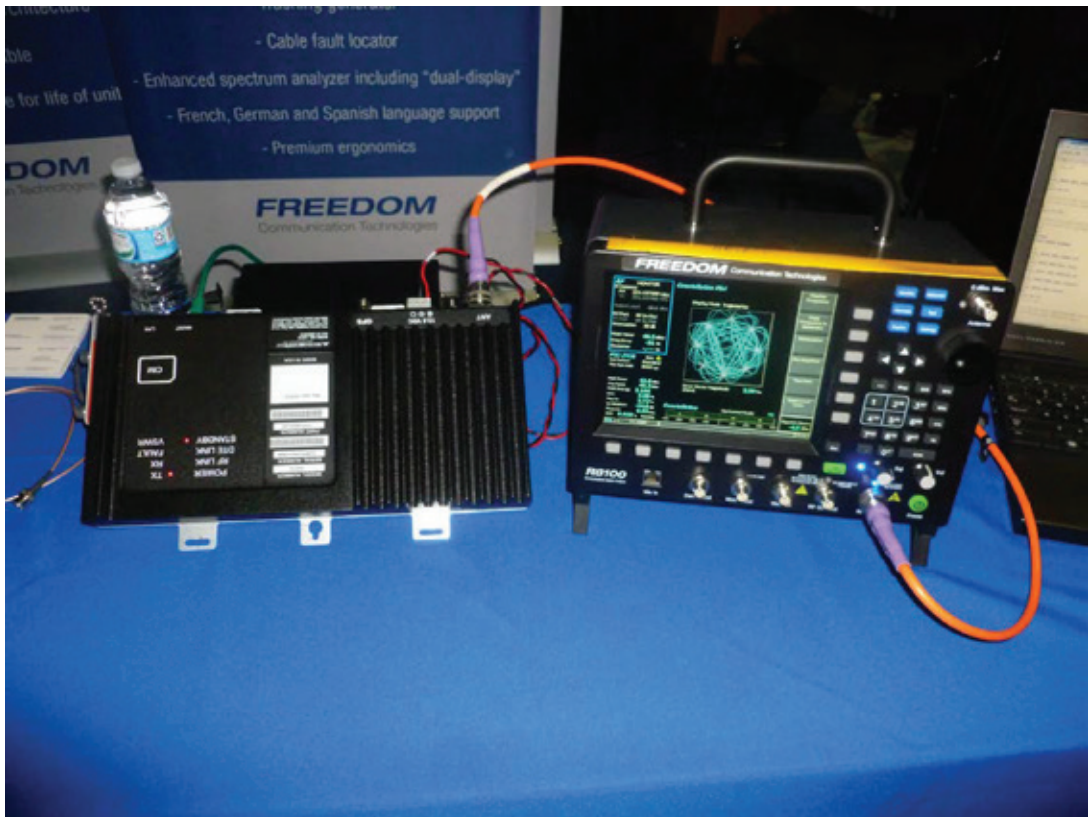
RF connection between Wayside and R8100
