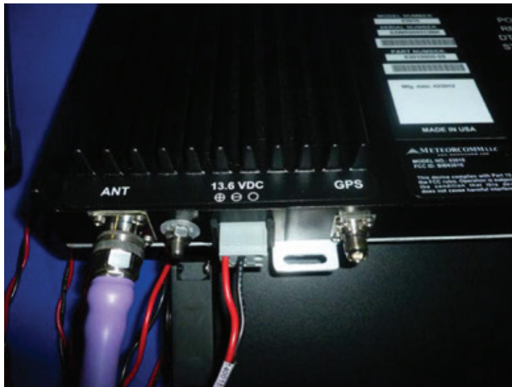
Power and Antenna connection on PTC wayside radio
