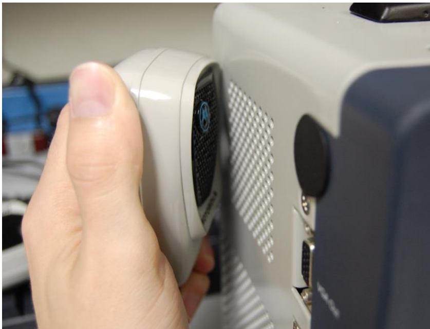
Figure 8-1. Place keyed radio next to analyzer speaker.
