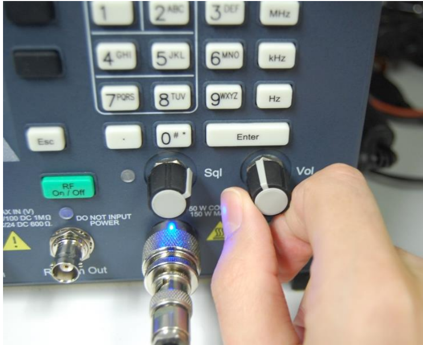
Figure 8-2. Adjust analyzer volume until about 4 kHz deviation is measured.
