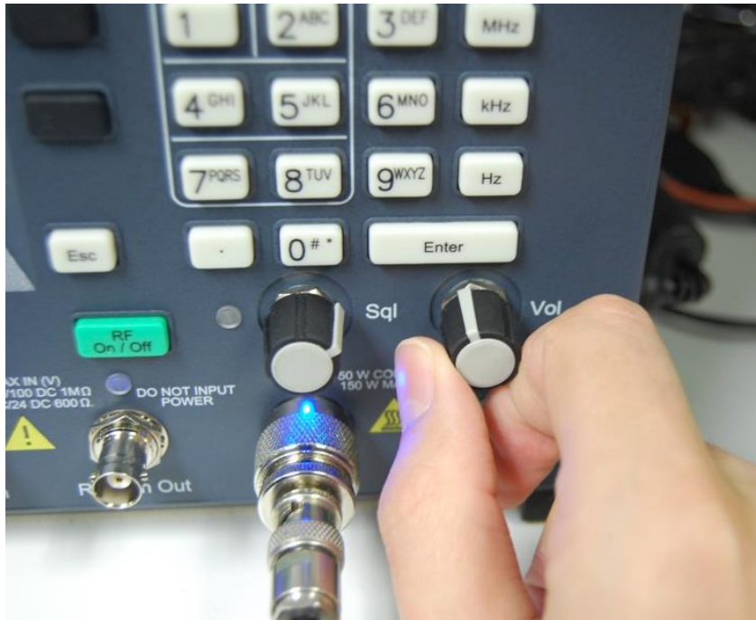
Figure 4-2. Adjust analyzer volume until about 60% rated system deviation is measured.
