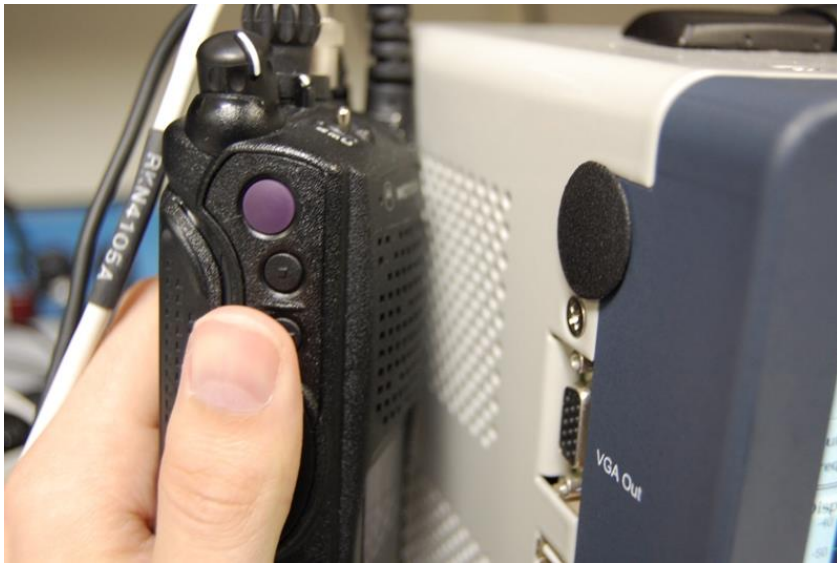
Figure 4-1. Place keyed radio next to analyzer speaker.
