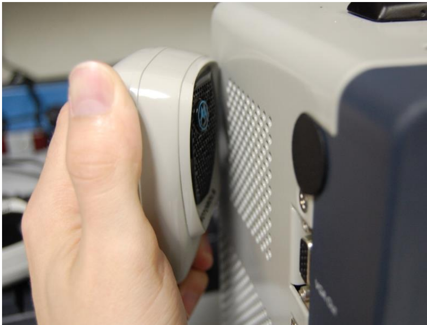
Figure 6-2. Place keyed microphone next to analyzer speaker.
