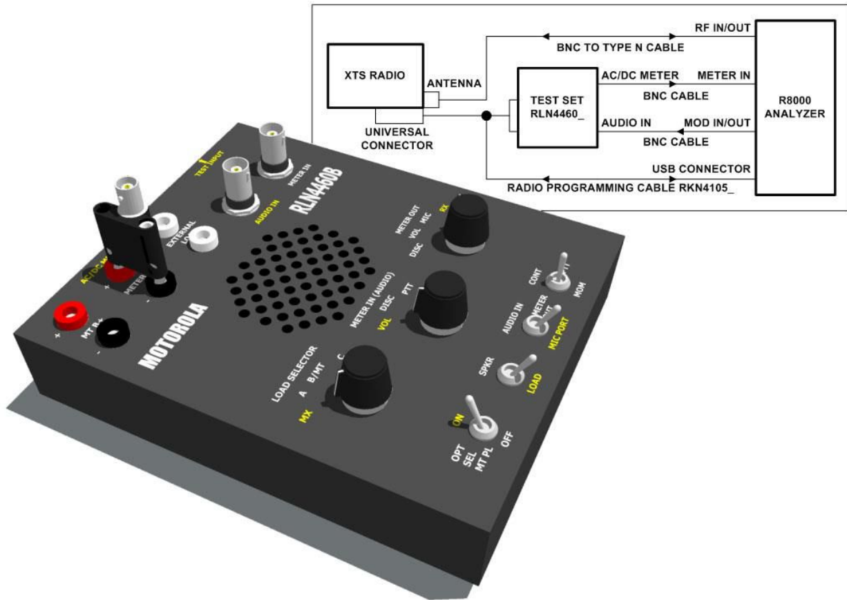
Figure 5-1. ASTRO® XTS™ Series Test Setup Diagram
