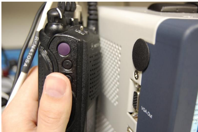
Figure 6-1. Place keyed radio next to analyzer speaker.
