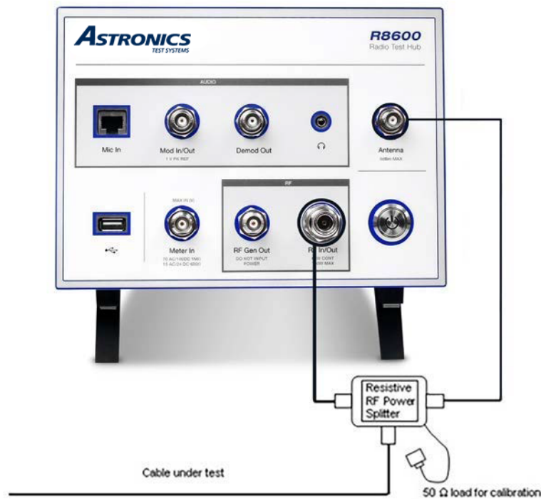
Figure 5.3-1 Connections for Cable Fault testing
