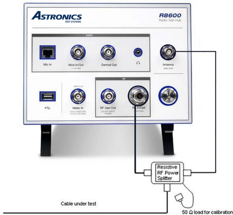
Figure 5.3-1 Connections for Cable Fault testing
