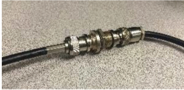
Normalize: calibrate out cable and adapter losses using a barrel connector
