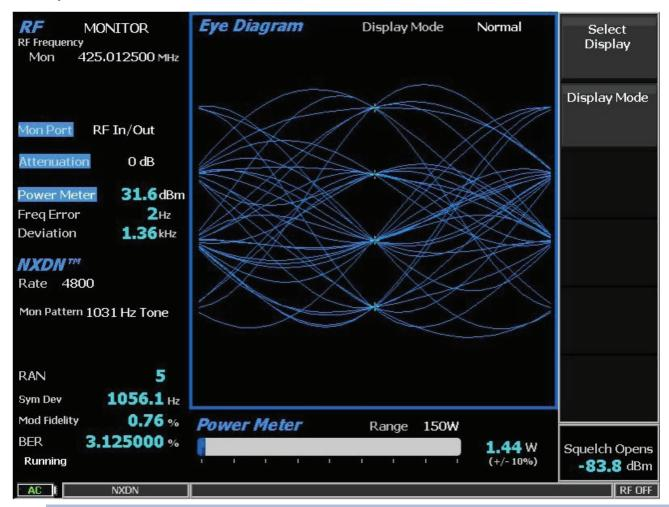
Note that the "Symbol Deviation Error %" and "Modulation Fidelity %" measurement fields display the quality of the radio's Digital Modulator.
