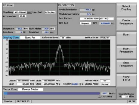
Note 1: The R8000 configuration and settings above may be saved as a "Preset". This avoids having to go through the setup procedure every time you need to conduct this test.
