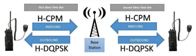
P25 Phase 2 voice channels are 12.5 kHz wide and contain two time slots. Each slot carries a separate channel of traffic. This means the portable/mobile radio is only transmitting 50% of the time.
