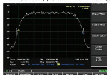
The Spectrum Analyser will be familiar as it is a copy on of the main Spectrum Analyser from the standard R8100. Only the functions applicable to TMO have been copied across,
