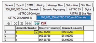
Once the TX frequencies are entered, the corresponding channel number is calculated. Alternately, you can enter the channel number and the frequency will be calculated. Remember the following formula:
