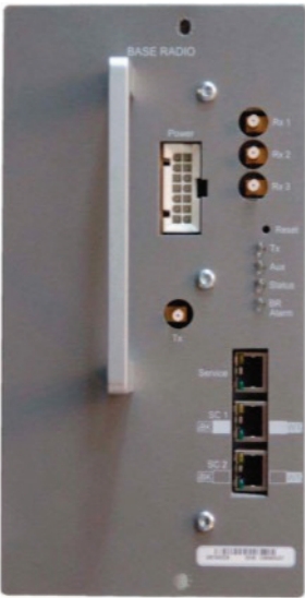
Base Radio – NOTE separate TX and RX ports
