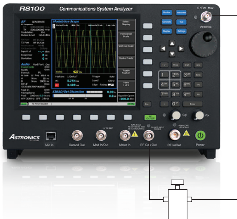
Figure 2 – Hookup to test a Pass-Reject cavity filter on the R8000 analyzer
