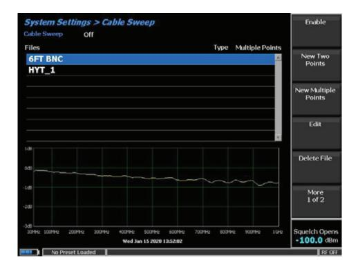
On the above screen the file "6FT BNC" data is shown in the graphic plot below the list.
