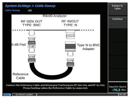
The screen asks the user to connect a reference cable between the Gen Port and the RF I/O port.
