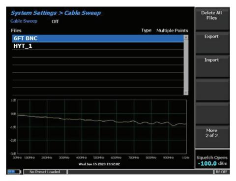
FCT-1017A Using the Cable Sweep functionality 8
