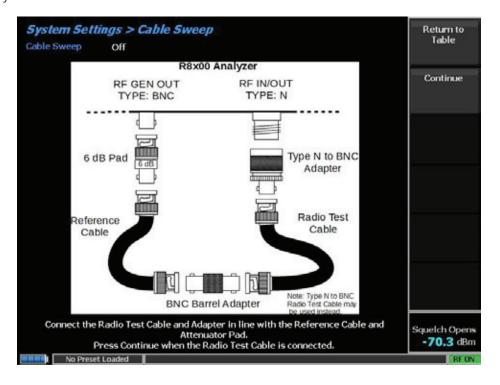
Now connect the "test cable" in line with the reference cable.
