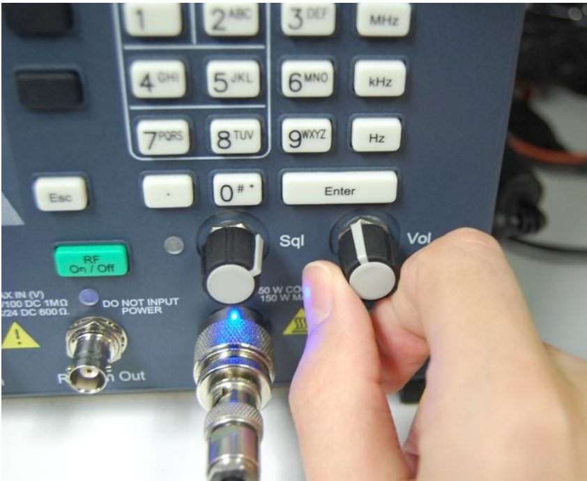
Figure 6-3. Adjust analyzer volume until about 60% rated system deviation is measured.
