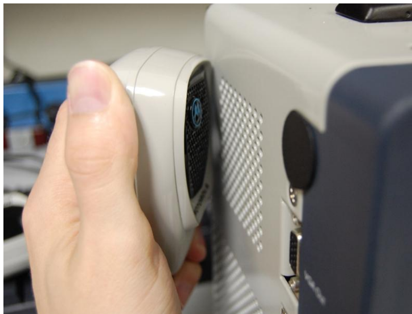
Figure 6-2. Place keyed microphone next to analyzer speaker.
