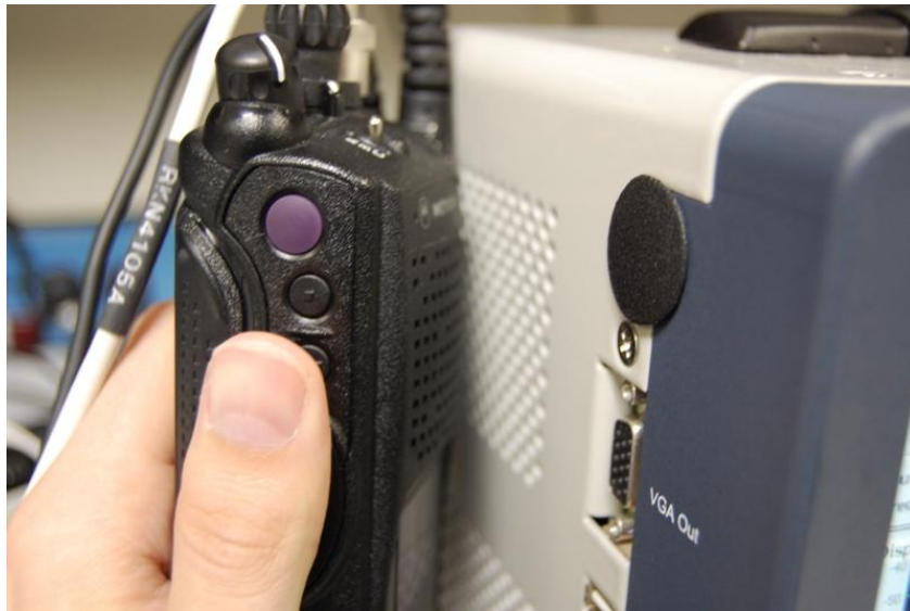
Figure 4-1. Place keyed radio next to analyzer speaker.
